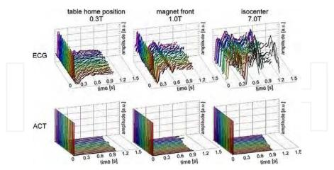
Fig. 10. ECG (top) and acoustic trigger signal (bottom) traces acquired at three different field strengths using the MRI scanners internal physiological signal processing unit. Severe signal distortion occurred in the ECG signal obtained at the magnet's isocenter, whereas the trigger signal derived from ACT remains undistorted
