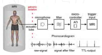
Fig. 9. Block diagram of acoustic cardiac triggering (ACT). ACT is free of interferences from electromagnetic fields and magneto-hydrodynamic effects, and provides a reliable trigger signal free of jitter even in the presence of free breathing.
