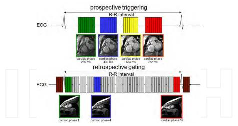
Fig. 1. Basic scheme of prospective triggering and retrospective gating in cardiac MRI using the electrocardiogram.
