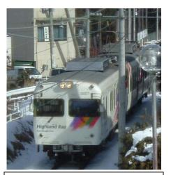
An electric train is just of example of a DC EMI source. Electric trains draw large amounts of current, which create a DC magnetic field, which can be a source of electromagnetic interference (EMI).
