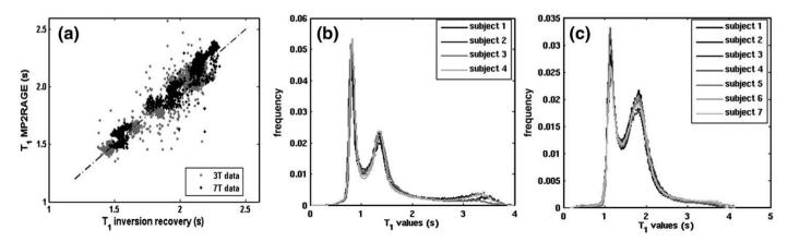
Fig. 7. (a) Pixel by pixel correlation of the T<sub>1</sub> maps obtained in a head phantom using the MP2RAGE and the IR-EPI at 3 T (grey dots) and 7 T (black dots). T<sub>1</sub> histograms of the entire brain after brain extraction at 3 T (b) and 7 T (c). Note the inter-subject reproducibility of the signal intensities and T<sub>1</sub> values using the sequence parameters detailed in Table 1.
