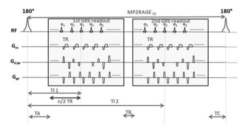
Fig. 1. Diagram of the MP2RAGE sequence. Inversion times  $Tl_1$  and  $Tl_2$  are defined as the time from the middle of the inversion pulse to the excitation corresponding to the center k-space line in the phase encoding in the slab selection direction. MP2RAGE<sub>TR</sub> is the time between two successive inversion pulses and TR is the time between successive excitation pulses in the GRE kernel, which is composed of n excitations.
