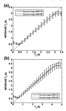
**Fig. 6.** Plots of the MP2RAGE  $T_1$  value estimated and their standard deviations using the optimized MP2RAGE parameters derived for 3 T (a) and 7 T (b) as a function of the real  $T_1$ . Black and light grey lines represent scenarios where the SNR of the second image is 10 and 50, respectively.
